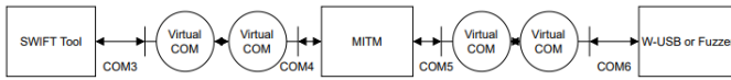
Fig. 17. Diagram of com0com virtual COM port connection layout for the MITM script.
